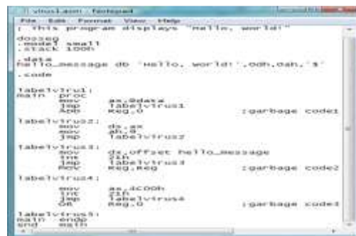
Figure 1: Assembly code of Virus File
